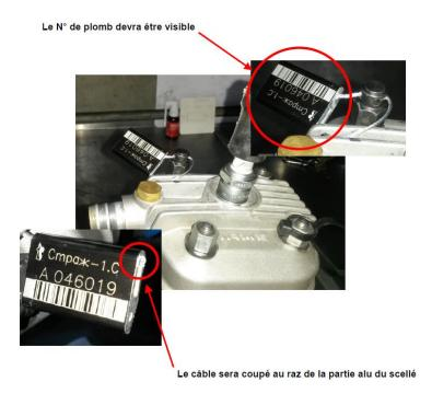
Don't forget to seal your engine and present your engine passport at the technical inspection.
